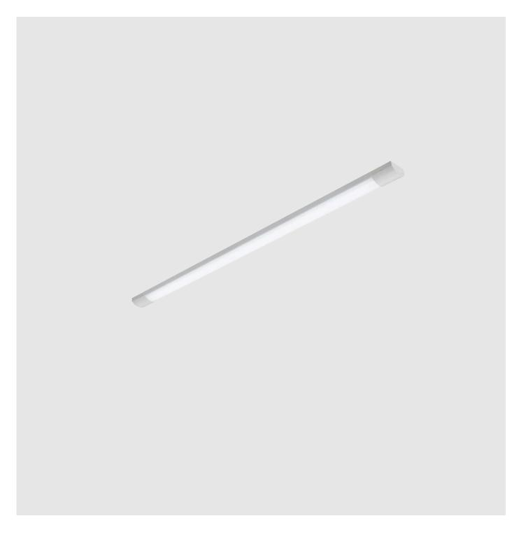
Prisma is a compact LED Batten with great versatility. It's tunable white option makes it ideal for any time of application, from commercial to residential. Ideally used for garages, store rooms and amenities. Prisma is available in 20W or 40W with powder coated aluminium body, polycarbornate diffuser and end caps.
