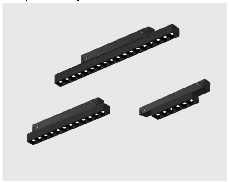
Dark Light is a DC48V recessed magnetic luminaire designed for precise and controlled illumination. Offering beam angles of 20°, 36°, and 48°, along with tunable white (2700K–5000K), the Dark Light adapts to various lighting needs. Compatible with DALI dimming, for smooth brightness control. Crafted from aluminum and Poly-Carbonate, and available in white or black, the Dark Light is a compact form, seamlessly integrating into modern architectural spaces with its magnet mounting system.
