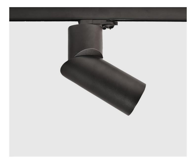
Elle features a two part cylindrical shaped housing in die cast aluminium, opal diffuser and an integral power supply with standard dimming for the 13W and optional dimming for the 20W version. As a ceiling, wall or track mounted fitting it can also be used as a directional spotlight. The Elle is a versatile fitting that is used in Residential, Retail, Hospitality and Commercial projects.
