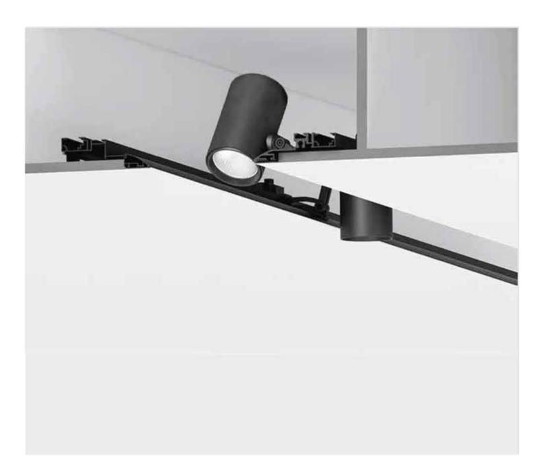
Cove is a profile system designed for recessing into coffers and ceiling or wall spaces. Made in die cast aluminium and using high powered COB LED's, the light source is recessed into the luminaire housing for reduced glare and visual comfort. It is ideal for use in Retail and Commercial applications to provide a clean and open space feel.
